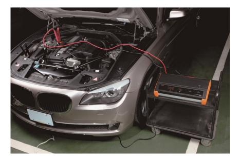
The Voltage Stabilizer must be able to maintain the set voltage regardless of the current draw created by actions such as fans and other components operating during the programming procedures.
